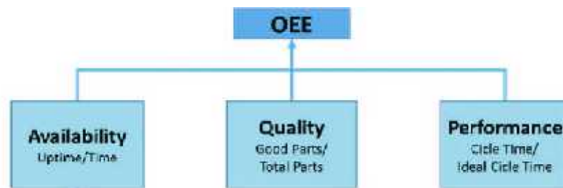
Fig 1. OEE indicator components.
