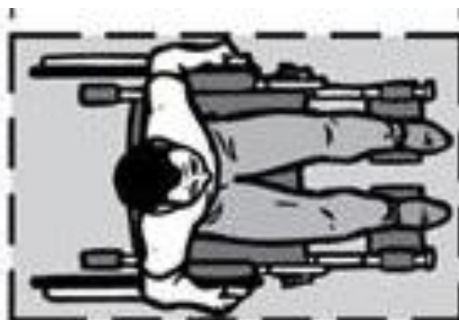
Fig. 6. Plan view showing an outline of a clear floor space of 80 cm by 135 cm
