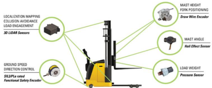
Fig. 4. Example of sensors used in an AGV structure
