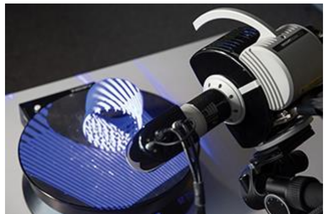
Fig. 2. 3D scanner based on structured white light, produced by Hexagon [5]
