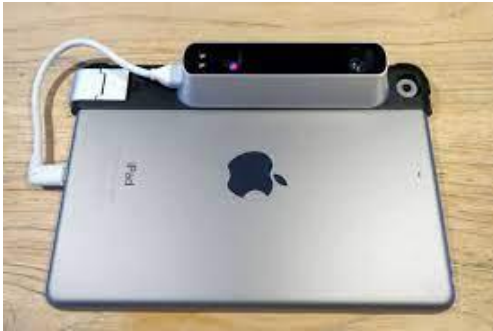
Fig. 3. 3D scanner based on photogrammetry, produced by Occipital [7]
