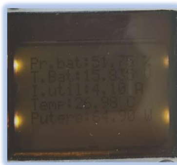
The real-time display of battery parameters (Voltage, Current, Power consumption, remaining battery capacity, battery temperature) can be found both at the software level (in the UMC interface) and hardware level (by displaying key parameters using a display (Fig. 5)).
