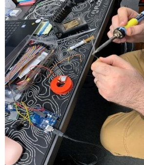
Fig. 4-5 Working steps for soldering the GSM module
