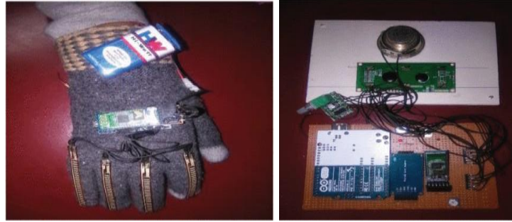
Fig. 2. Gesture Conversion Device Comprising Two Parts: Glove and Station[3]
