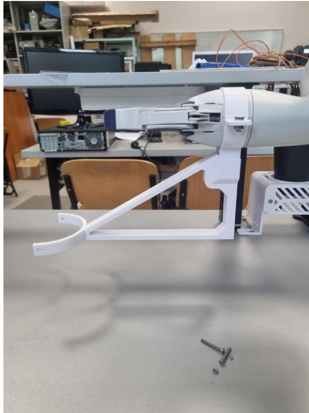
Fig. 8. The mount assembled on the robotic arm.
