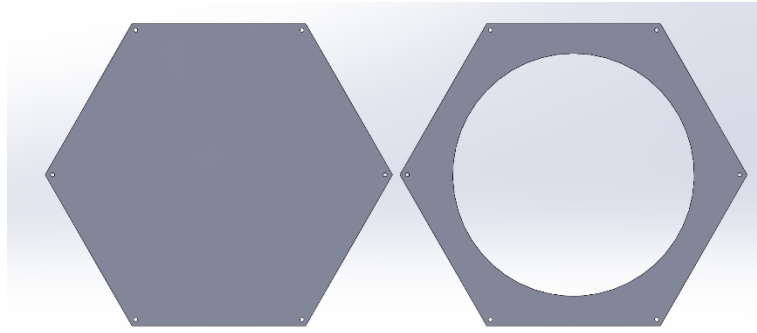
Fig.7 Top plate (left) and bottom plate (right)
