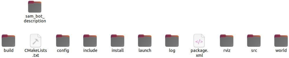
Fig. 2. "sam_bot_description" working environment and its contents
