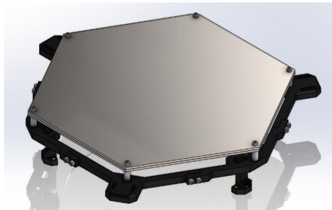
Fig.6 Subassembly of the printing bed
