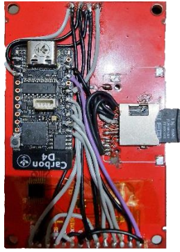
Fig. 6. The command circuit of the display
