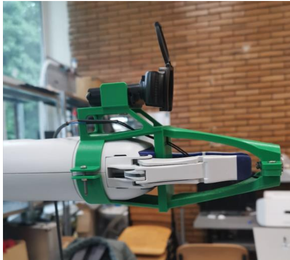
Fig. 9. Assembly of articulated robotic arm and end-effector
