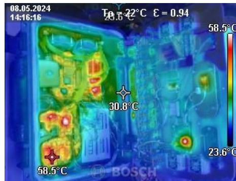
Fig.17 Thermal view of the UMC
