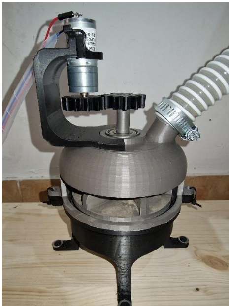
Fig. 8. Sand mechanism subassembly
