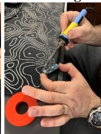
Fig. 6-10 Arduino board soldering steps
