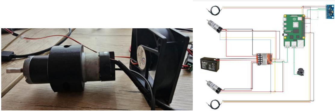
Fig.5. The placement of the fan and the final connection diagram.
