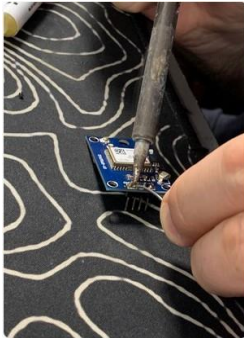
Fig. 2-3 Working steps for soldering the GPS module
