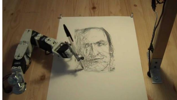
Fig .1. Drawing made by a robot with 3DOF
