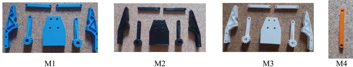
Fig. 4. Actual specific components of the product Gripper GR 01.00 of material M1, M2, M3, M4 respectively
