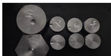
Fig. 6. Indentations in steel plates
