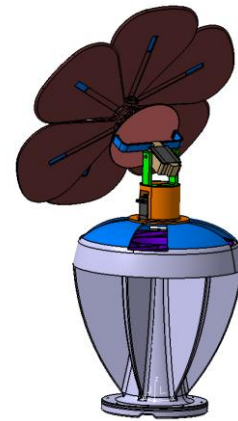
Fig.6. Integration of the Protection and Solar Tracking Mechanism into the Device
