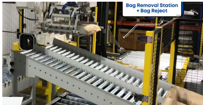
Fig. 1 Conveyor removing non-compliant bags
