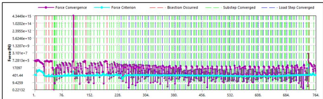
Fig. 6. Convergence of Iteratively Applied Forces
