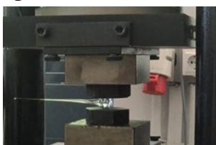
Fig. 5. Borosilicate drop during testing
