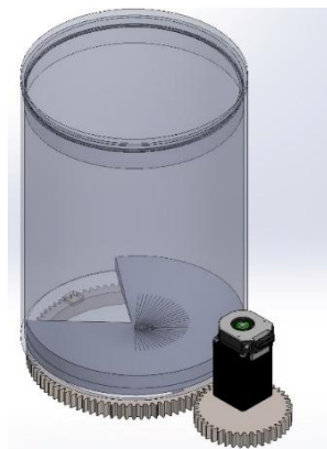
Fig. 7. Storage and dosing assembly
