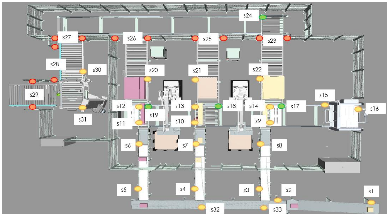
Fig. 3 Location of the sensors in the robotic cell
