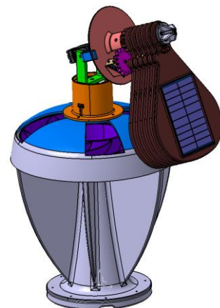
Fig.7. Protection of the Photovoltaic System through Solar Panel Folding
