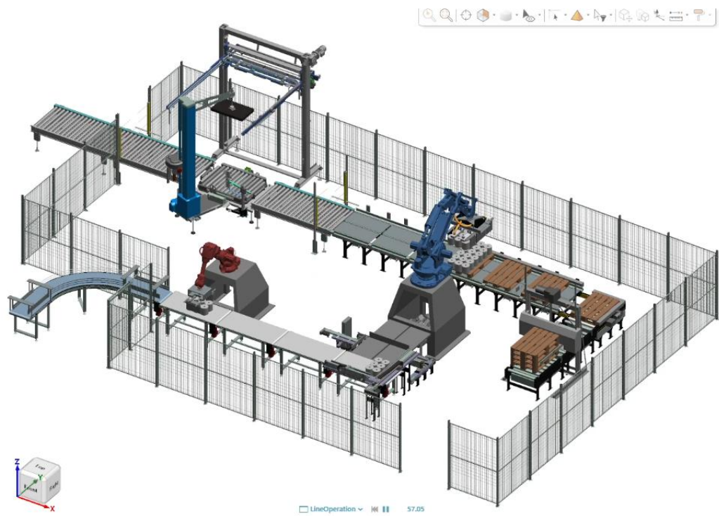
Fig.13 Palletizing object layers by the 4-axis robot
