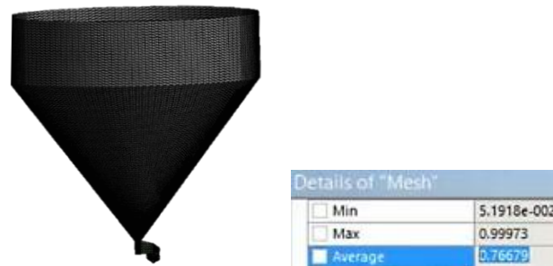
Fig. 2. Face meshing and element quality
