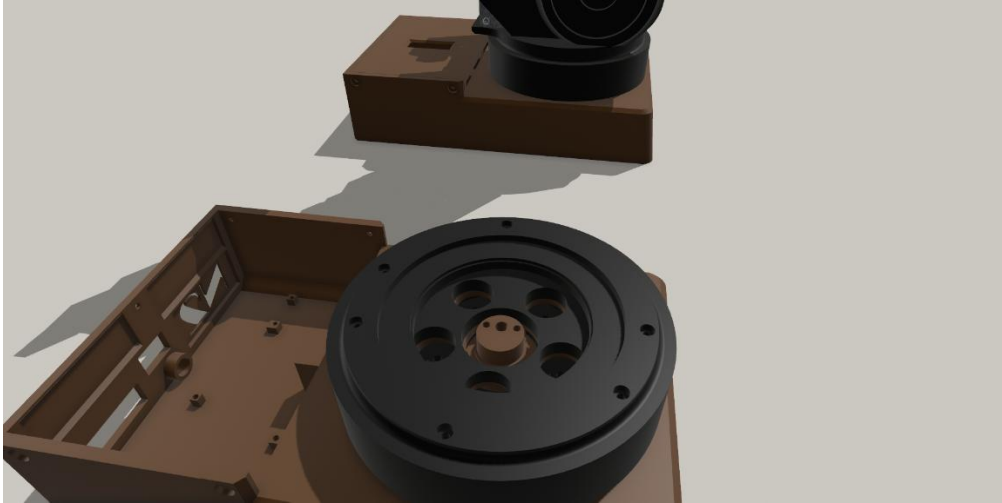
Fig. 9. N2 – Cycloidal Gearbox System (1:10) For J1
